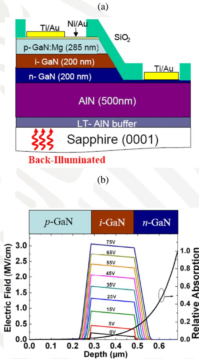
Figure:1 (a) Schematic structure of GaN-based APD and (b) Electric field across the device.
